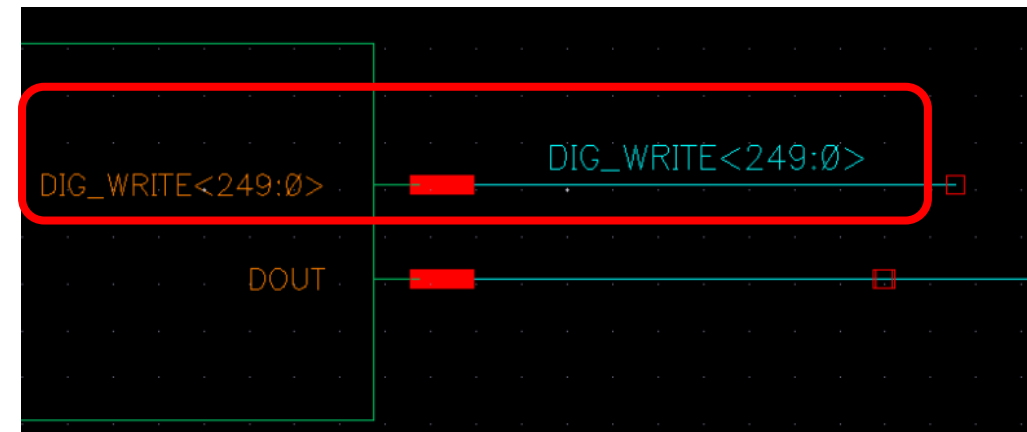
Testchip block with large bus (250 bits)
